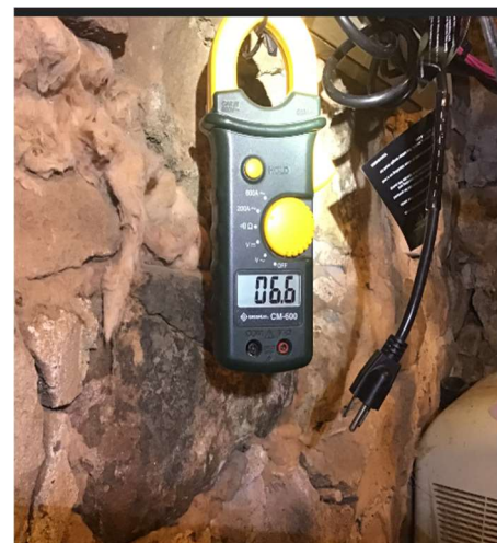
Figure 12: Current under normal load
